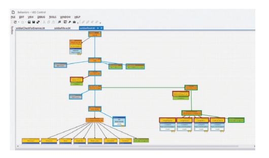
designed for creating behaviors for individual soldiers or vehicles, as well as behaviors for higher military echelons up to a company level. The simulation of these AI entities is provided by VBS4. Using the VBS Simulation SDK, developers can extend AI behavior capabilities and interact with external systems.
